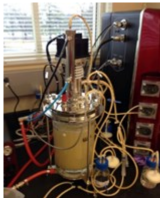
Figure 2. Butyric acid fermentation setup.
